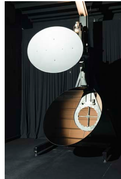
Photometric Measurements - Goniophotometer with rotating mirror
